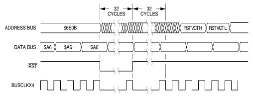
Figure 13-16. Wait Recovery from Internal Reset
