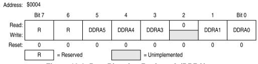
Figure 12-2. Data Direction Register A (DDRA)
