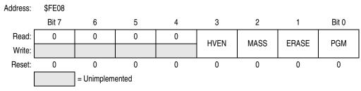
Figure 2-3. FLASH Control Register (FLCR)
