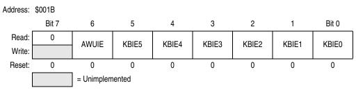
Figure 9-4. Keyboard Interrupt Enable Register (KBIER)
