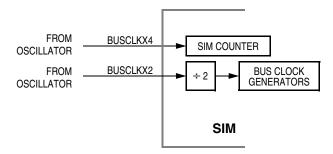
Figure 13-2. SIM Clock Signals
