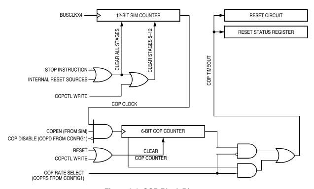
Figure 6-1. COP Block Diagram
