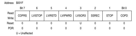
Figure 5-2. Configuration Register 1 (CONFIG1)
