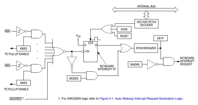
Figure 9-2. Keyboard Interrupt Block Diagram
