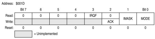
Figure 8-3. IRQ Status and Control Register (INTSCR)
