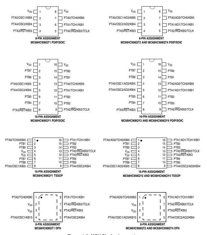
Figure 1-2. MCU Pin Assignments
