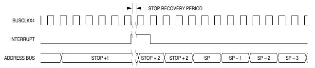
Figure 13-18. Stop Mode Recovery from Interrupt
