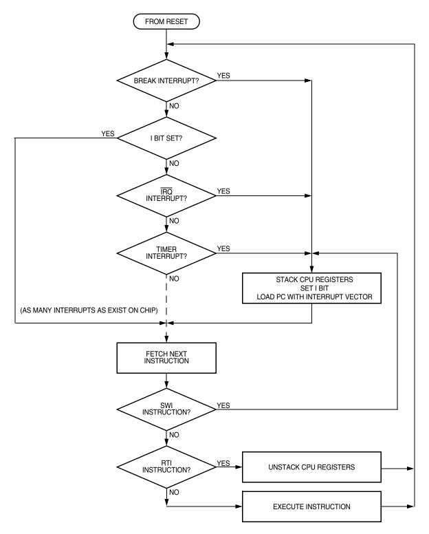
Figure 13-7. Interrupt Processing
