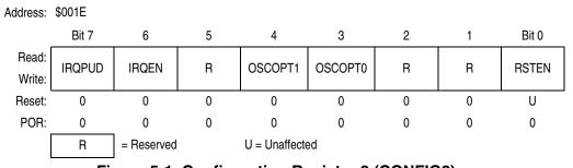
Figure 5-1. Configuration Register 2 (CONFIG2)
