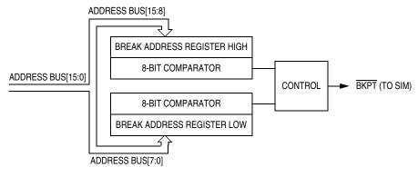
Figure 15-2. Break Module Block Diagram
