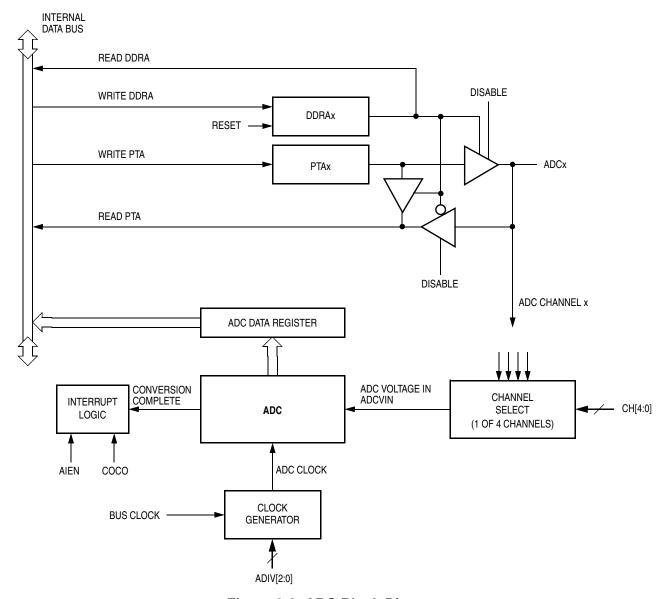
Figure 3-2. ADC Block Diagram
