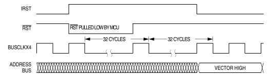
Figure 13-4. Internal Reset Timing
