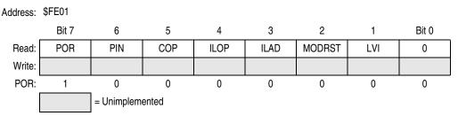
Figure 13-19. SIM Reset Status Register (SRSR)
