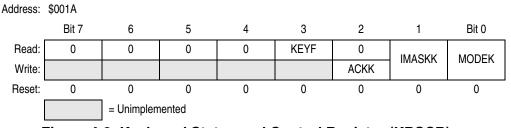
Figure 4-3. Keyboard Status and Control Register (KBSCR)
