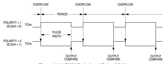
Figure 14-3. PWM Period and Pulse Width
