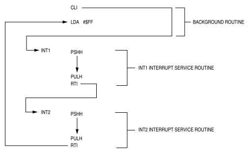
Figure 13-10. Interrupt Recognition Example
