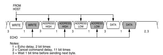
Figure 15-16. Write Transaction
