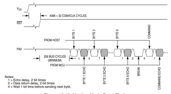
Figure 15-18. Monitor Mode Entry Timing
