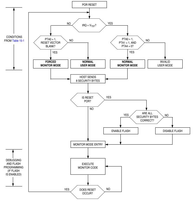
Figure 15-9. Simplified Monitor Mode Entry Flowchart
