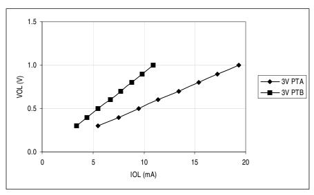
Figure 16-6. Typical 3-Volt Output Low Voltage versus Output Low Current (25°C)
