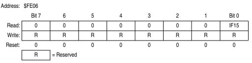
Figure 13-13. Interrupt Status Register 3 (INT3)
