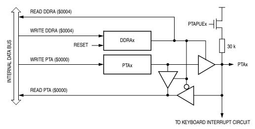
Figure 12-3. Port A I/O Circuit
