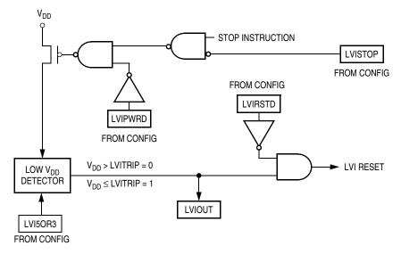
Figure 10-1. LVI Module Block Diagram
