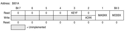
Figure 9-3. Keyboard Status and Control Register (KBSCR)
