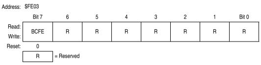
Figure 13-20. Break Flag Control Register (BFCR)
