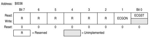
Figure 11-4. Oscillator Status Register (OSCSTAT)
