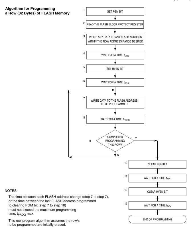
Figure 2-4. FLASH Programming Flowchart
