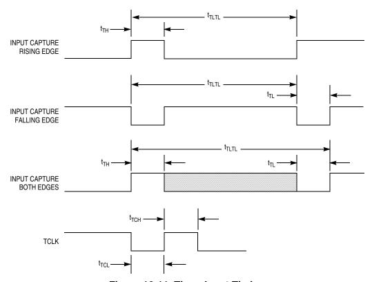
Figure 16-11. Timer Input Timing
