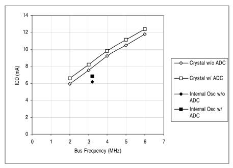
Figure 16-9. Typical 5-Volt Run Current versus Bus Frequency (25°C)
