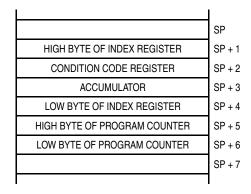
Figure 15-17. Stack Pointer at Monitor Mode Entry
