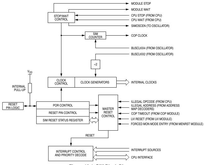
Figure 13-1. SIM Block Diagram
