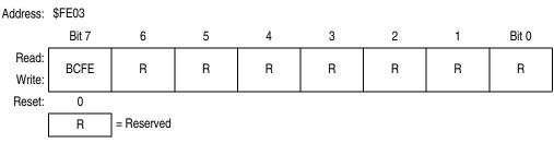
Figure 15-8. Break Flag Control Register (BFCR)
