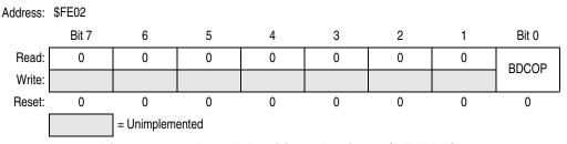
Figure 15-6. Break Auxiliary Register (BRKAR)
